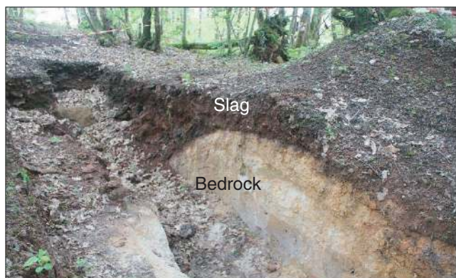
Figure 11. Structure of the slag heap with the slag overlying a siderolithic bedrock at a slag heap located at Saint-Vincent sur L'Isle test site in Dordogne (France). The GPS coordinates of the test site are longitude 0°53'17.9" and latitude 45°13'56.4". The ditch shown on the picture is located slightly north from the geophysical survey.
