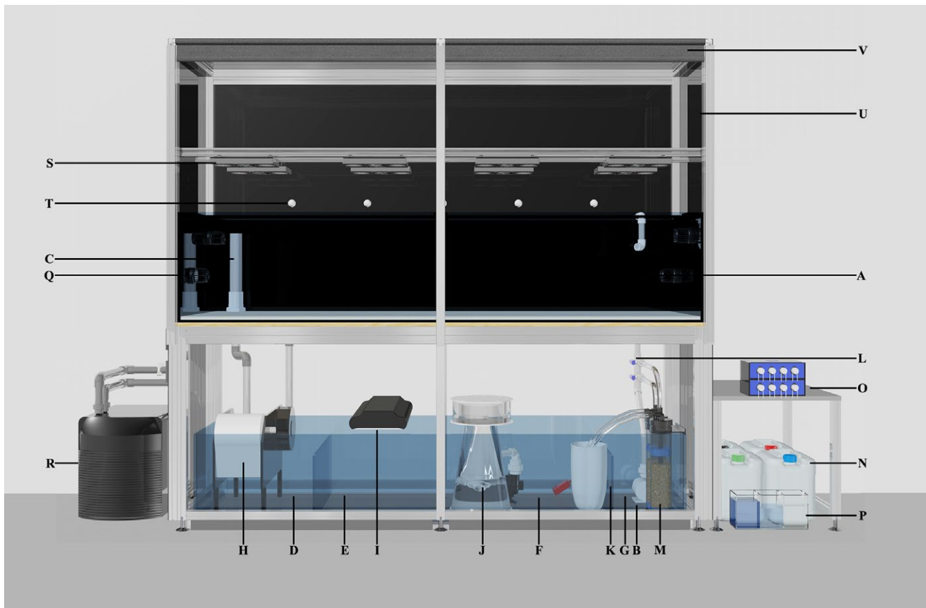
FIGURE 1 Mesocosm setup: (A) 780 L broodstock aquarium, (B) main drive pump, (C) 40 mm polyvinyl chloride (PVC) stand pipes, (D) mechanical filtration section of sump, (E) algae refugium, (F) protein skimming section of sump, (G) main drive pump section of sump, (H) E200 PowerRoll filter, (I) wave point luminar, (J) protein skimmer, (K) baffle, (L) 32 mm PVC inlet, (M) fluidized reactor, (N) Triton Base elements CORE 7, (O) four channel peristaltic pump, (P) multi chamber container for individual element corrective dosing, (Q) aquarium chiller, (R) Radion XR30W Pro LED light, (S) lunar LED, (T) black mdf panel fitted into an aluminum frame, (U) integrated blackout blind
