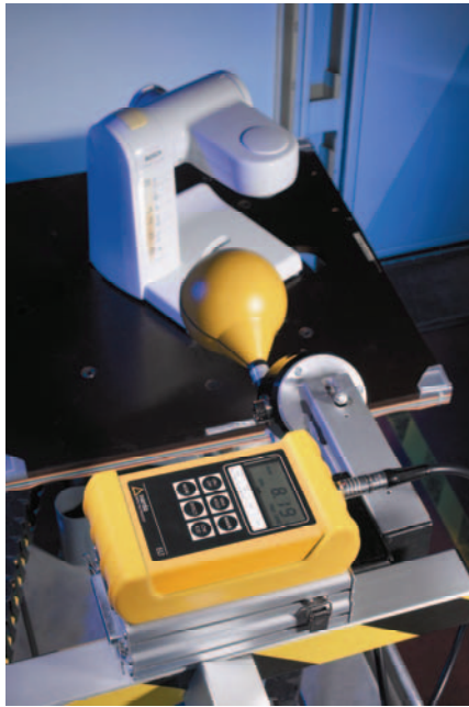
Fig.34. An example of a search coil magnetometer used for testing the electromagnetic compatibility (with permission of Narda Company)
