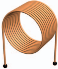
Fig.1. The simplest sensor of magnetic field in form of a coil
