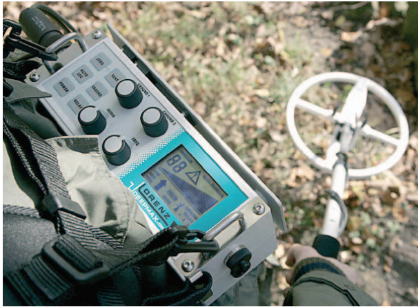
Fig. 39. An induction search coil as a tool for detection of metal objects (with permission of DCG Detector Center)
