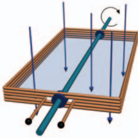
Fig. 19. The sensor of a DC magnetic field with a rotating coil
