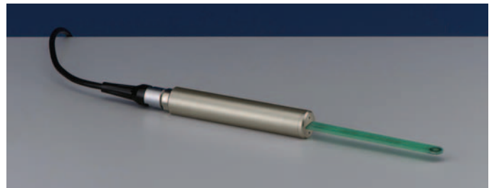
Fig.17. An example of the coil sensor used in a digital fluxmeter of Brockhaus
