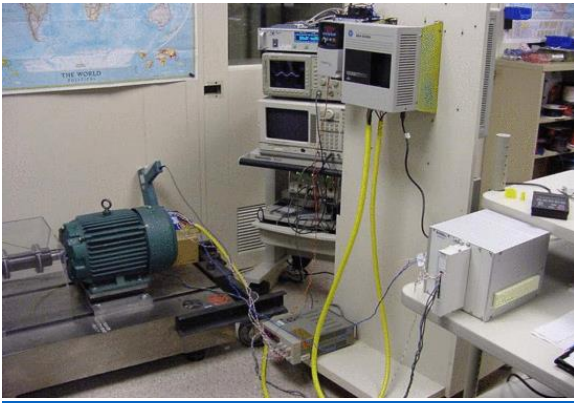
Fig. 4. Laboratory test setup for the 5-hp induction motor and data acquisition.
