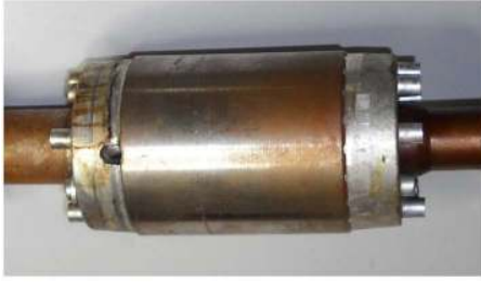
Fig. 5. Rotor featuring a broken bar.
