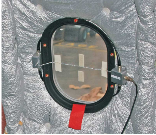
Fig. 2. Photograph of a window sensor. Two twisted wires form the central bar. The boxes provide connections and termination of the coaxial cables that act as outer perimeter of the figure-eight. The cables are mostly laid in a region of low magnetic flux, between fuselage and the top rim of the window pane mounting flange.
