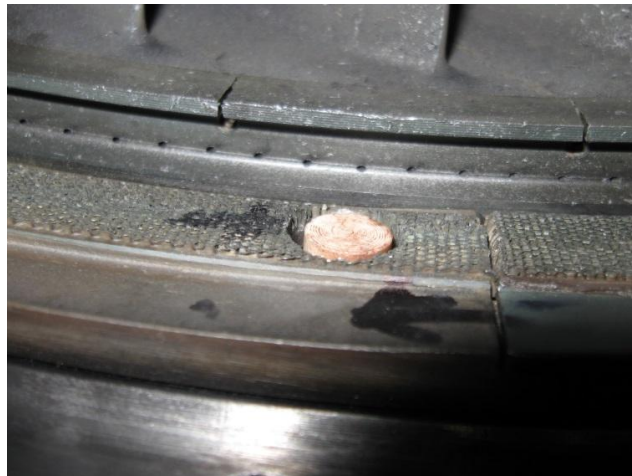
Fig. 2. Ceramic head of the sensor fitted into the casing of HPT
