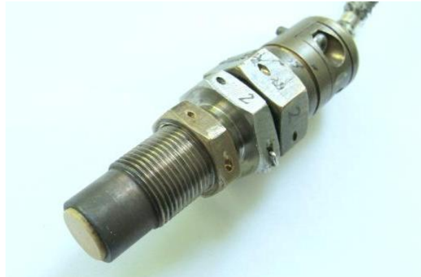
Fig. 1. The sensor after 60 hours testing in the a gas turbine
