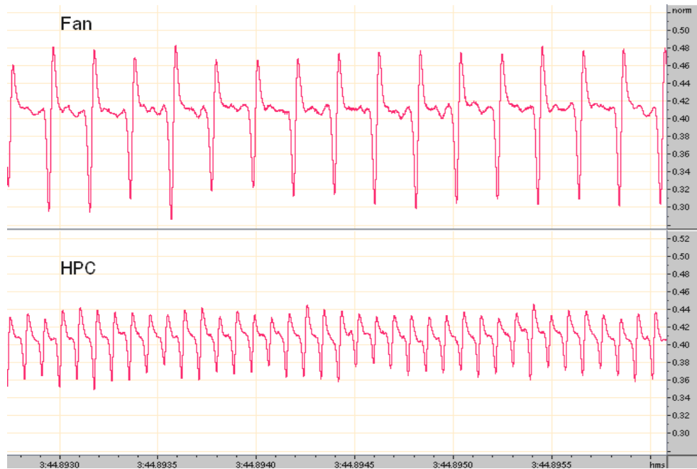
Fig. 3. Fan and compressor sensor output signal sampled at take-off speed
