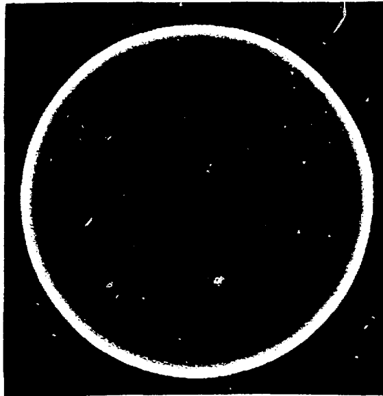
Fig. 18. Reconstruction with beam-hardening correction.
