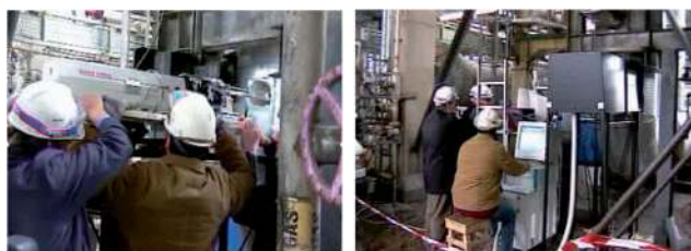
Fig. 6 LIBSGRAIN project: mounting of the laser at the plant for pipe analysis (left) and mapping of steel composition (right).
