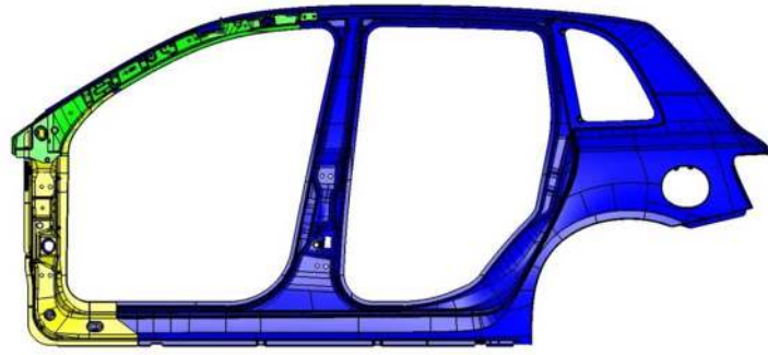
Figure 4. Bodyside components assembled in the case studies
