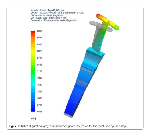
of its relatively large size (about 200 mm) and the loadings, the blade unscrews as illustrated on Figure 5, where one can appreciate the deformed geometry in color with respect to the initial configuration in gray. A maximum displacement of 3.86 mm is observed at the end of the structure.
