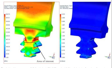
Fig. 6 Von Mises stress map [MPa] with the LATIN-PGD method (left) and deviation from the reference in percent [%] (right)
