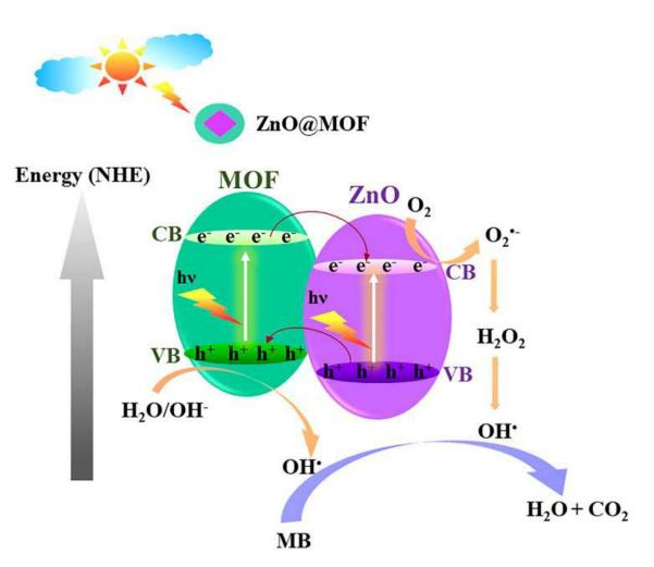
**Figure 2.** Photocatalytic mechanism of ZnO@MOF-46(Zn). Proposed reaction mechanism over ZnO@MOF-46(Zn) for photodegradation [82].
