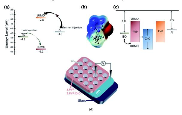
**Figure 5.** (a) Energy level diagram of the devices that are based on PVP. (b) The electrostatic potential (ESP) of the molecule as determined using DFT. (c) Illustration of the energy bands of the ITO/PVP:ZnO/Al device. (d) Schematic structure of resistive random-access memory (RRAM) device based on polyvinylpyrrolidone (PVP) and PVP:PVP:zinc oxide nanoparticle (ZnO NP) active layers [217].
