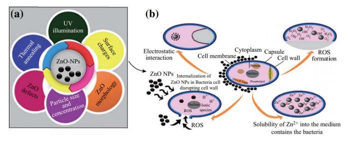
**Figure 1.** (a) An impact of key ZnO NPs parameters on the antibacterial response and (b) correlation between the several potential mechanisms of ZnO NPs antibacterial activity, such as ROS production,  $Zn^{2+}$  release, internalization of ZnO NPs into bacteria, and electrostatic interactions [34].
