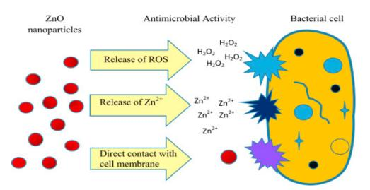
Figure 4. The mechanism of water disinfection by ZnO NPs [183].
