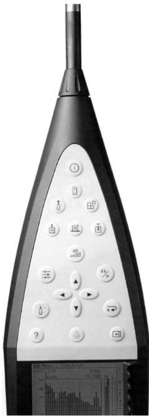
FIGURE 3-2 Sound level meter. This meter is a handheld modular precision sound analyzer system. (By permission of Brüel and Kjaer.)
