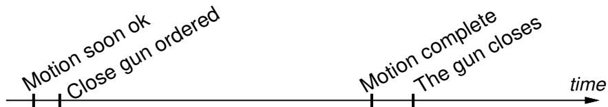
Figure 8.3 Timing for stop of motion and start of welding.
