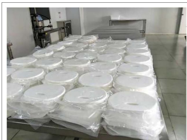
FIGURE 9 | BC-based raw materials for face mask. Reproduced with permission from Hainan Yeguo Foods Co., Ltd (2020).
