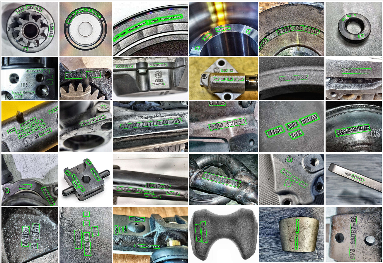
Fig. 7. Some multi-oriented detection examples on the MPSC dataset using RFN. Five styles of metal parts text are listed in five rows to illustrate the effectiveness of our method for multi-oriented text detection.
