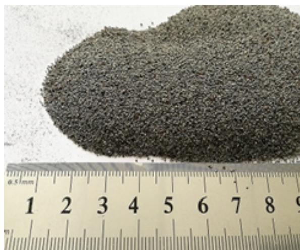
Figure 1 – Fly ash of Pavlodar thermal power plant-1
