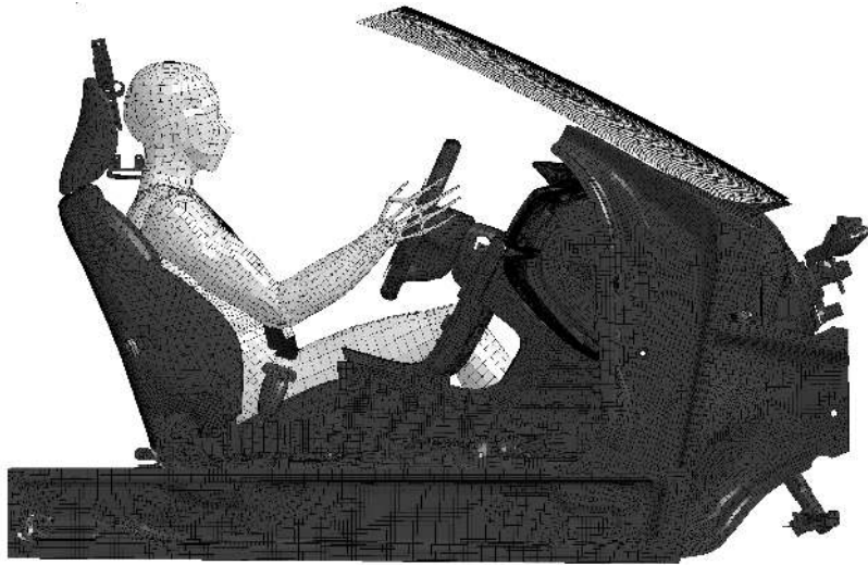
Figure 4.3: SAFER AHBM model positioned in full interior model for a crash simulations.
