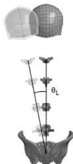
Figure 3.1: Lateral lean angle, \theta_L , between a vertical axis and the midpoint of the posterior inferior iliac spine and the centre of the T1 vertebral body.
