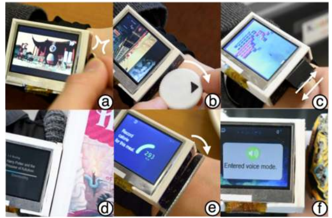
Figure 15. Inductive demo applications: (a) video player, (b) aircraft game, (c) brick breaker game, (d) audio book app, (e) fitness app, (f) setting voice mode app.
