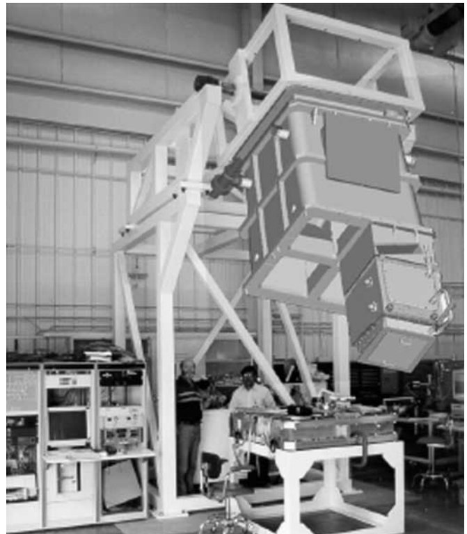
FIGURE 6. The full-scale FOA test stand (large steel structure in center of photo) was installed in the Bldg. 432 high-bay in March. A CAD representation of the FOA has been superimposed to illustrate the soon-to-be-installed hardware. The actual vacuum isolation valve is shown on a support stand at the bottom of the photo. (40-00-1098-2032pb01)
