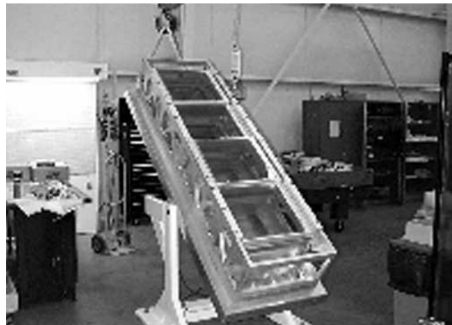
FIGURE 4. A single spatial filter lens assembly is shown above on the left. Four such assemblies are installed into a cassette, which has a strong back for stiffness/handling (shown on right). (50-00-1098-1989pb01 and 50-00-1098-1990pb01)
