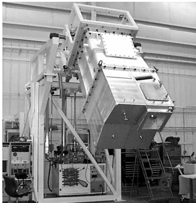
FIGURE 5. Prototype FOA hardware being assembled in the high bay of Building 432. (40-60-1198-2260pb01)
