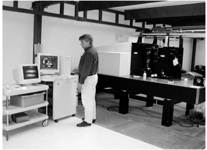
Final metrology on a 24" Zygo interferometer (provided by Corning)
