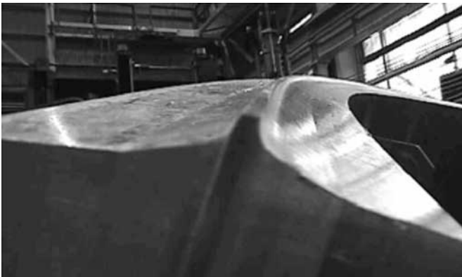
FIGURE 5. Shown is the radiused weld prep that has been machined on one of the target chamber sections. (40-00-1098-2033pb01)
