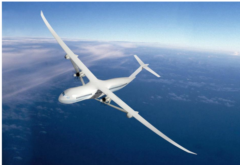
Figure 3. Boeing SUGAR Truss-Braced Wing (TBW) Aircraft Concept
