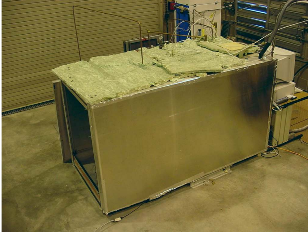
FIGURE 3. PHOTO OF FUEL TANK SPECIMEN IN THE AIRCRAFT COMPONENTS FIRE TEST FACILITY
