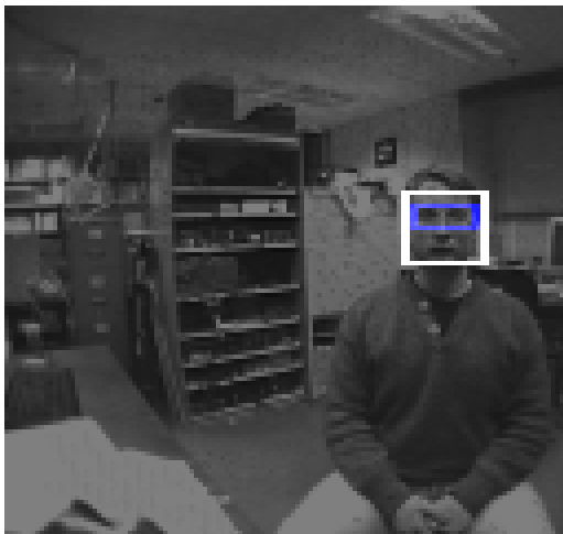
Figure 6. An example face in a cluttered environment. The 128x128 grayscale image was captured by the active vision system and then processed by the pre-filtering and ratio template detection routines. One face was found within the image, and is shown outlined.
