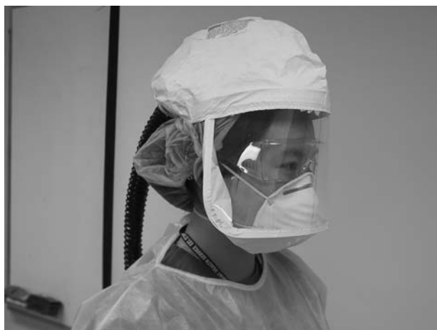
FIGURE 1 A lightweight headpiece is connected to the powered air purifying respirator (PAPR) system via a tube
