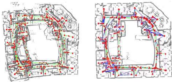
Fig. 8. Intel without front-end loop validation. Our system can identify correct loop closures and compute a posterior map from within a single integrated Bayesian framework (right); the typical front-end loop validation has been replaced with a k + 1 mixture component containing the k best laser scan matches (based purely on overlap) plus a null hypothesis. In this experiment, we used k = 5 . For reference, the open-loop trajectory of the robot is given on the left.
