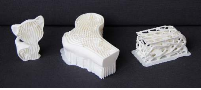
Fig. 19: FDM printed replicas of some models generated by our formulation.
