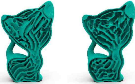
Fig. 9: As the minimum thickness increases from left to right, the wall-like structures are more and more replaced by truss-like structures.
