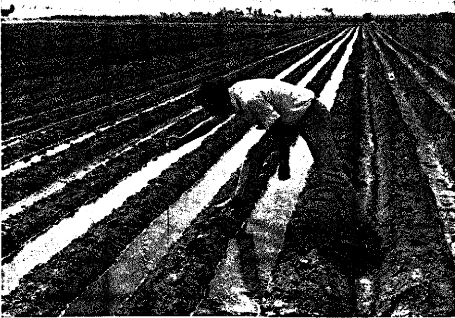
FIG. 7. Depth of water h and the width T taken with a tape measure.
