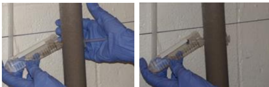
Figure A-3.1: Core sampling of the filter bed using a plastic syringe to push the media.
