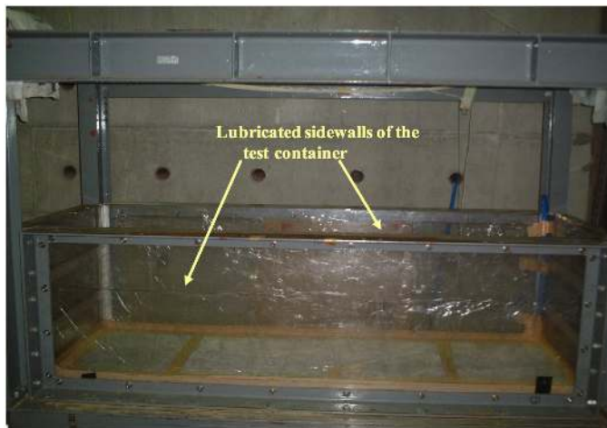
Figure 1: Lubricating the sidewalls of the test container before forming the sand bed
