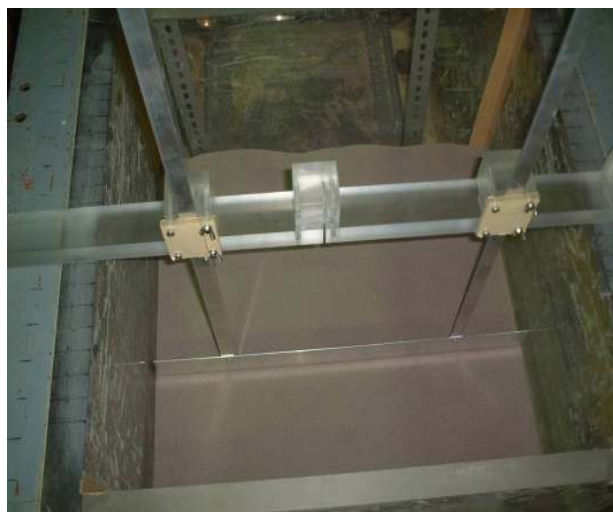
Figure 4: Manually-controlled instrument to form flat sand layers in the test container
