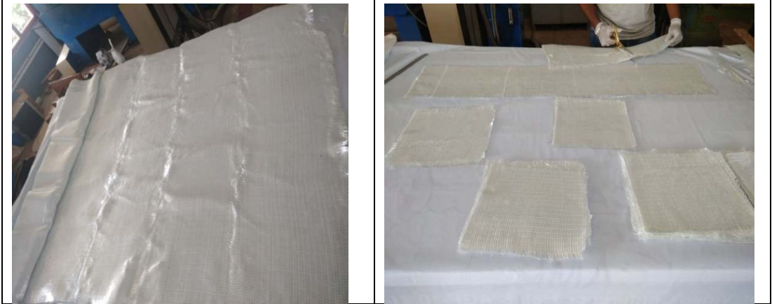
Fig. 1 - Cutting woven glass fabric in to required mould/ mold dimensions
