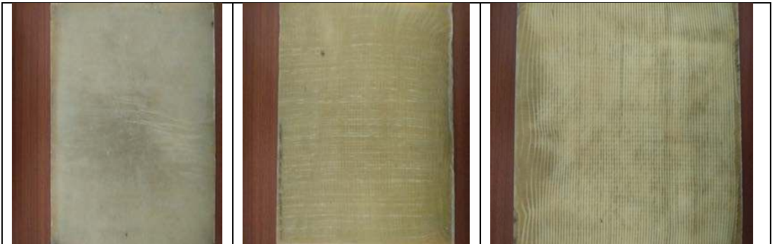
Fig. 2(a, b, c) - Fabricated 7 M, 0^\circ-90^\circ , +45^\circ/-45^\circ GWFE composites
