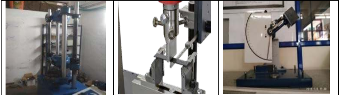
Fig. 3(a, b, c) - Experimental setup of Tensile, Compression, Flexural and Impact tests
