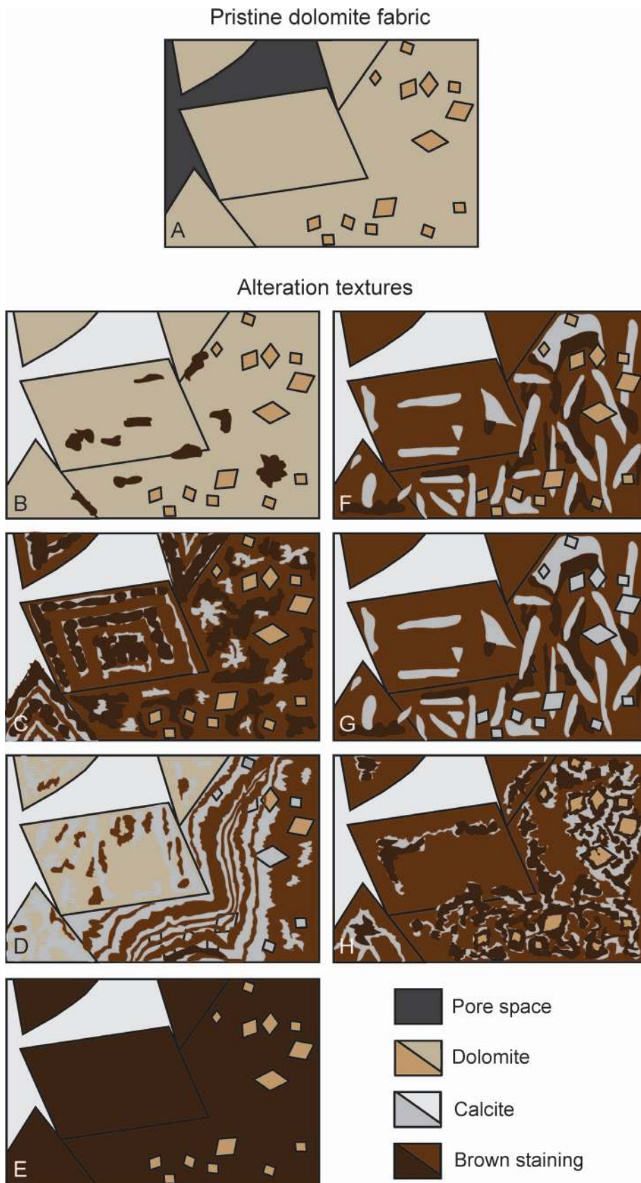
FIG. 9.—Alteration textures of fault-related dolomite fabric. A) Pristine dolomite fabric with orange brown dolomite rhombs representing D1 and gray-brown coarser dolomite representing D2. B) Well-preserved texture with coarse iron-rich D2 dolomite crystals that can display a few brown patches at crystal borders or growth zones or cleavages. C) Brown and calcitized zonations and darker and lighter brown irregular mottles in the coarse D2 crystals. D) Small thin colloform brown bands and calcitized zones. Part of the D2 dolomite may be better preserved; also D1 crystals may or may not be calcitized. E) Dark brown or reddish brown homogeneous large zone in D2 dolomite, whereas D1 dolomite rhombs may be preserved. F) Reddish brown fishbone-like calcitized texture with preserved small D1 rhombs. G) Reddish brown fishbone-like calcitized texture with calcitized small D1 rhomb relicts. H) Mottled dark brown pattern in partially calcitized reddish brown zone and some preserved D1 dolomite rhombs.
