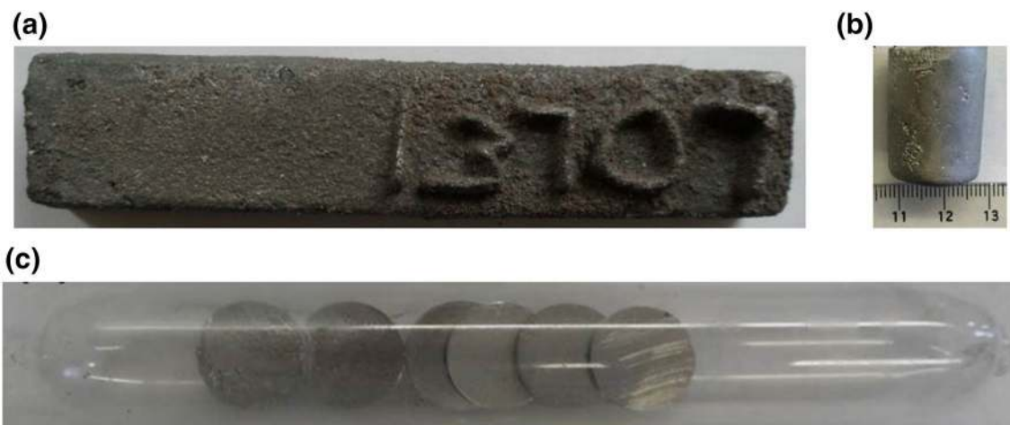
Fig. 1 a Keel bar selected for the experiment. b Example of a recast sample solidified at a controlled rate. c Typical encapsulated samples for controlled cooling from the homogenization temperature
