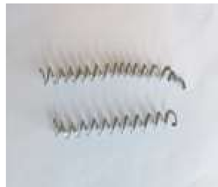
Fig. 6b. Washer type helical chip formation
