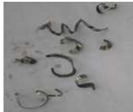
Fig. 6a. Arc chip formation
