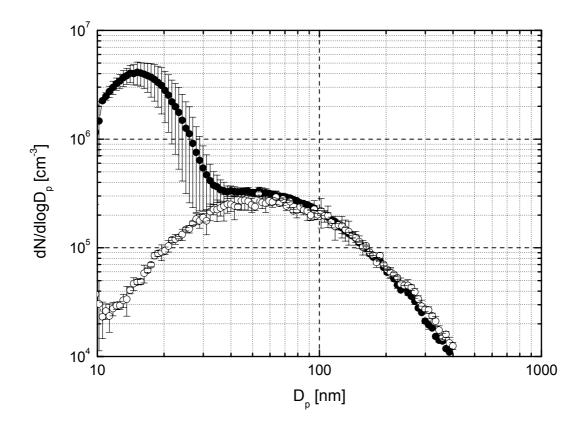
Figure 3: A typical SMPS number-size distribution spectra where a nuclei mode was observed with LS diesel (full circles) and no nuclei mode was observed with ULS diesel (open circles). Each distribution represents the mean of three SMPS scans under the same conditions with the error bars as shown. This example is for Bus 5 in Mode 8. Both distributions have been corrected for dilution.
