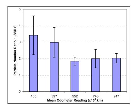
.Figure 5 : Ratios of total particle number emission rates with LS and ULS diesel fuel in all four operational modes as a function of the odometer readings of the buses. The buses have been classed into five groups according to the odometer readings and the histograms show the mean ratios for each group.
