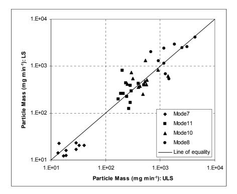
Figure 1 : Particle mass emission rates with LS diesel vs ULS diesel fuel. Each point represents a given mode and bus. The symbols differentiate the four operational modes and the straight line represents equality.
