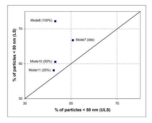
Figure 4 : Mean percentage of particles smaller than 50 nm in the SMPS number-size scans at each operational mode with LS diesel fuel plotted against the same quantity with ULS diesel fuel.
