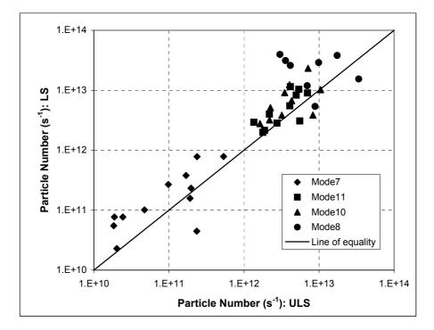
Figure 2 : Particle number emission rates with LS fuel vs ULS fuel. Each point represents a given mode and bus. The symbols differentiate the four operational modes and the straight line represents equality. particle number concentrations are in the size range 8 to 400 nm.
