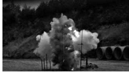
(b) The cylindrical charge of L/D = 1 , showing clear asymmetry on the axis, and large effect on the axis
