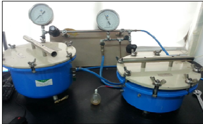
Fig 2. 15 bar Pressure Plate Extractor.
