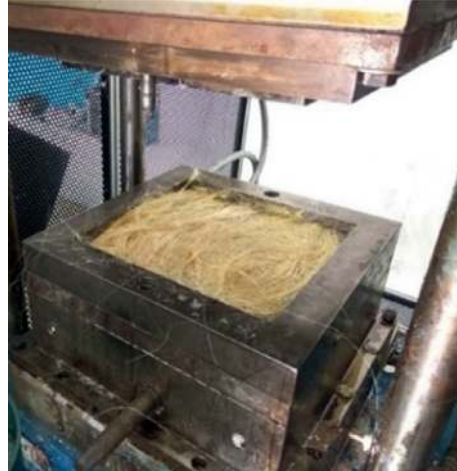
FIGURE 1: Preparation of samples with a hot compression method.
