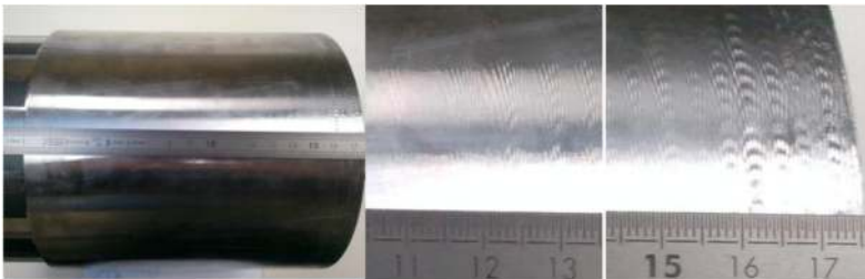
Fig. 5. Surface of the tube after the last tool pass
