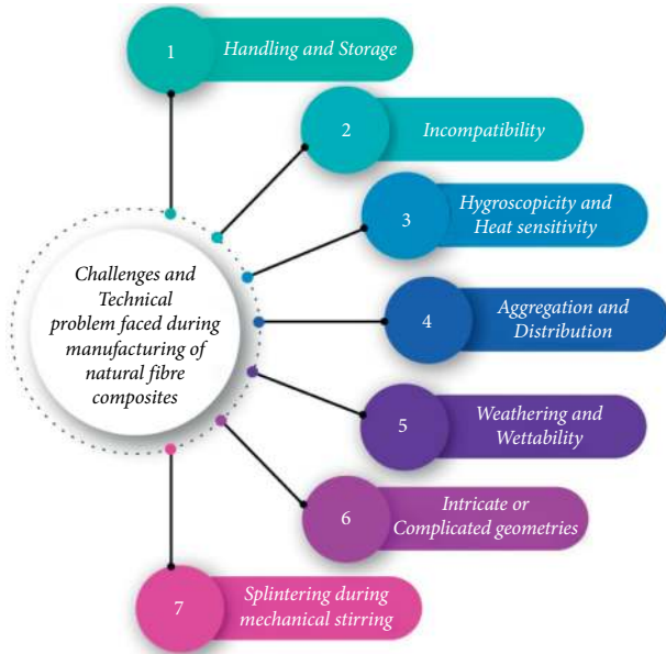
FIGURE 1: Challenges and technical problems faced during fabrication of natural fibre composites.
