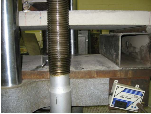
(a) Draw wire transducer details
