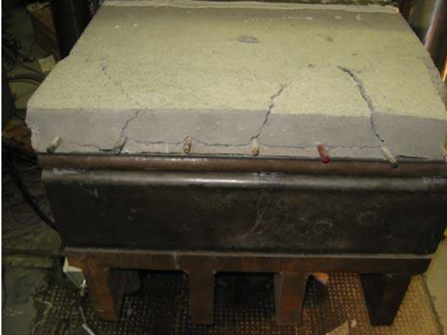
(c) Specimen 6x2 after testing
