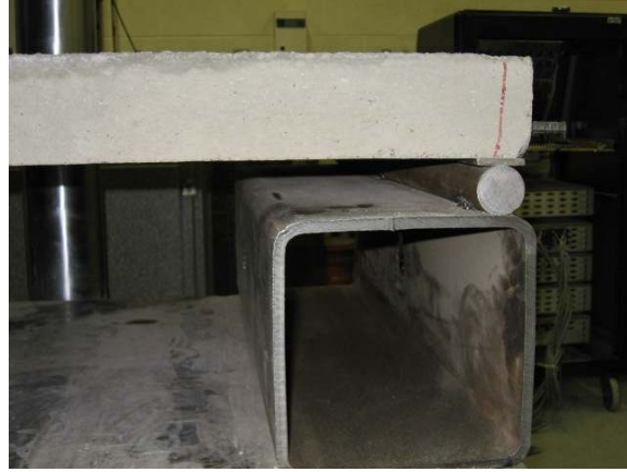
(b) Details of the support
