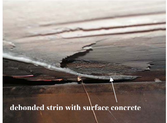
(b) Specimen 1x4 after testing
