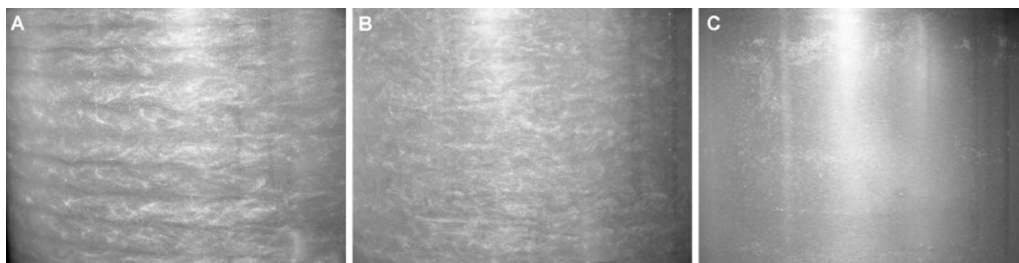
FIG. 1. Photographs of the flow at Re=3.6 \times 10^3 . Left, A: only the inner cylinder rotating. Middle, B: counter-rotating cylinders. Right, C: only the outer cylinder rotating. The flow structure is visualized using microscopic mica platelets (Pearlessence).
