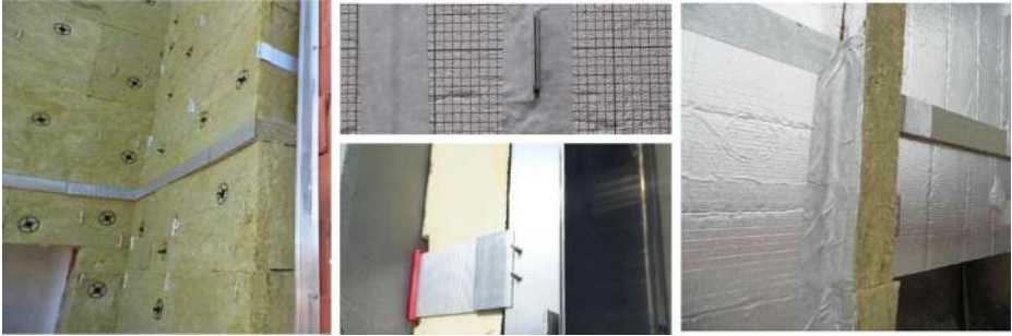
Figure 2. Stone wool (left: Sample 1-2), PIR (middle Sample 3-5), Phenolic foam (right: Sample 6-7).
