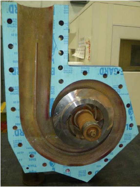
Figure 1: Split line detail of casing with the impeller in place on its carrier for the Test Rig.
