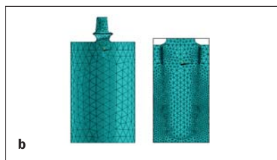
Figs 2a to 2d Schematic drawing showing (a) an osseointegrated implant embedded in bone and (b to d) a finite element model with mesh generation for (b) a 1-piece implant, (c) an internal-hex implant, and (d) an external-hex implant.
