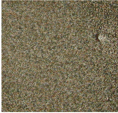
Figure 2. Optical texture by POM for CBO7O.Py after the TSDC thermal treatment. Typical nematic domains within the amorphous material can be appreciated together with some scarce crystalline nuclei.
