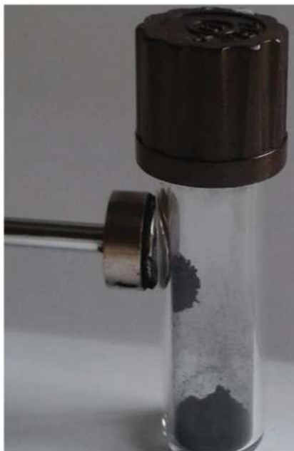
Figure 3. Image of the magnetic separation of one of the synthesis products. Each sample powder under the action of the permanent magnet shares into two parts, magnetic and nonmagnetic one, respectively.
