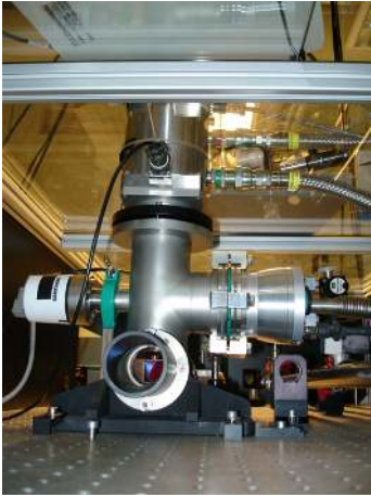
Figure 3.2. Cryogenically cooled 25 \times 25 \times 20 \text{ mm}^3 Ti:Sapphire crystal, pumped with 7 J at 532 nm. Transverse lasing is inhibited by absorbing carbon sheets surrounding the amplifying medium.
