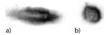
Figure 6.11. CR39 imprints of proton beams, shown on the same greyscale: a) controlled shot into a vertical fibre of the nylon mesh, and b) a shot on a microsphere. Both beams have a vertical full divergence angle of \approx 30^\circ .
