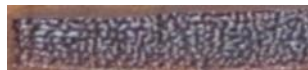
Figure 19. Appearance of sintered surface PMS-1 (x2), sintering modes P=30 W, t=200 °C, V=3000 mm/min, S=0.1 mm.
