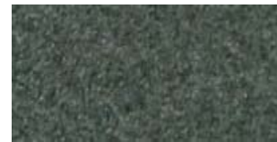
Figure 24. Appearance of sintered surface DSK-F75 (x2), sintering modes P=10 W, S=0.15 mm, V=300 mm/min, t=200 °C.
