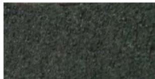
Figure 23. Appearance of sintered surface DSK-F75 (x2), sintering modes P=10 W, S=0.15 mm, V=300 mm/min, t=26 °C.
