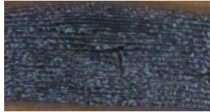
Figure 9. Appearance of sintered surface PMS-1 (x2), sintering modes P=30 W, t=200 °C, S=0.3 mm, V=200 mm/min.
