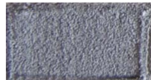
Figure 18. Appearance of sintered surface PA-4 (x2), sintering modes P=10 W, t=26 °C, V=1000 mm/min, S=0.2 mm.
