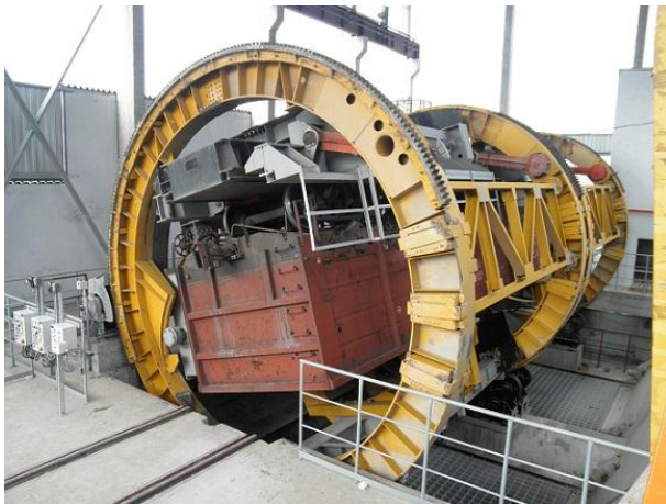
Fig. 7. Stationary rotary car dumper VRS-93, VRS-93-110
