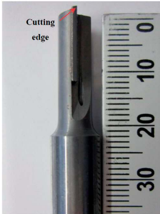
Figure 3. PCD tool used with two straight flutes.
